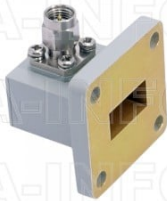
51WCASM_Cu Right Angle Rectangular Waveguide to Coaxial Adapter 15-22GHz WR51 to SMA Male
