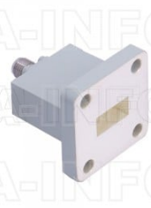
51WECAK_Cu Endlaunch Rectangular Waveguide to Coaxial Adapter 15-22GHz WR51 to 2.92mm Female
